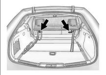
The net can also be mounted to the tethers on the back of the rear seats when the seats are upright.
